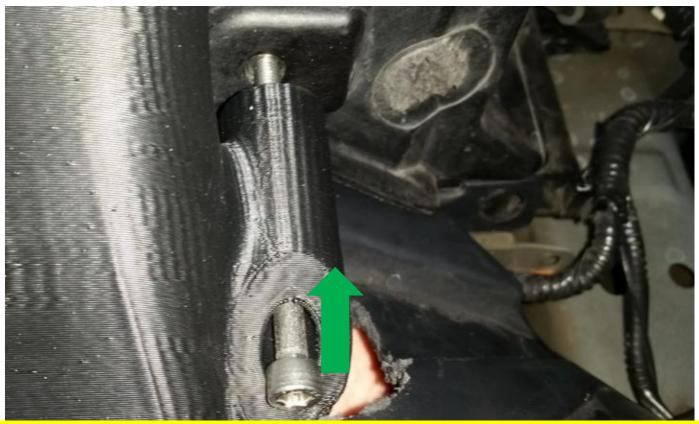
Push the bolt in and begin threading by hand as you support the nut on the backside.
