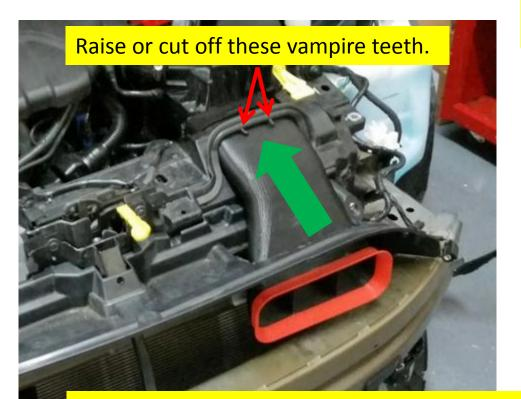
Apply a small film of grease or dish soap to the last inch of duct
