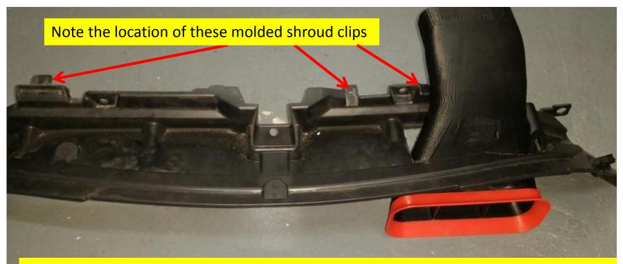
Place the shroud and intake back on the car as a unit, do not put the push-clips back in yet. You will need the shroud to be a little loose so you can work. (You may want to clip it in using the tabs that are molded on the back of the shroud)
