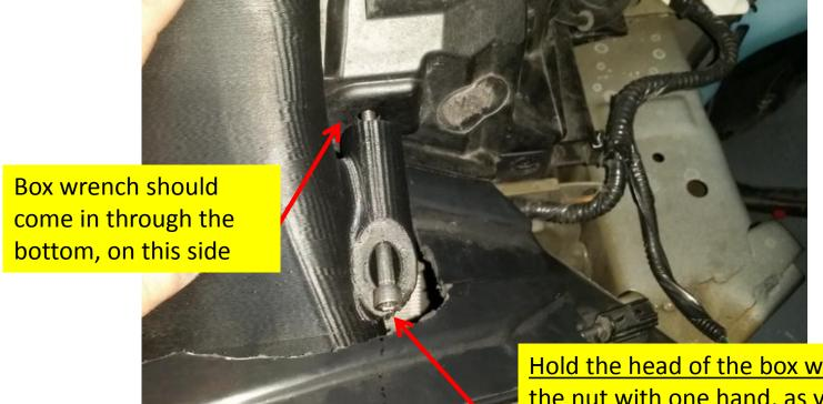
Hold the head of the box wrench over the nut with one hand, as you tighten the allen wrench with your other hand.
